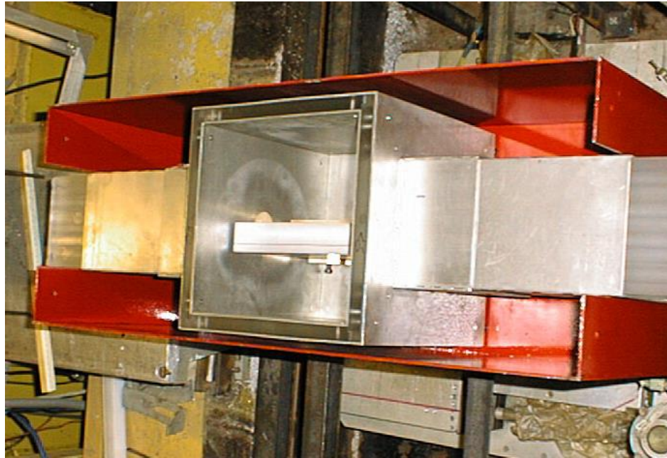
Photo: The spin manipulator with a sample holder in the process of its assembly at the neutron reflectometer NR-4M (beam 13, WWR-M reactor, Gatchina) for measurements with 3D-polarization analysis with the sample in zero field, in the absence of spin precession.
