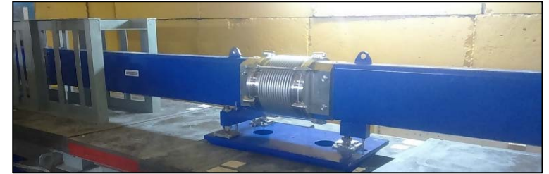
Focusing part of neutron guide
