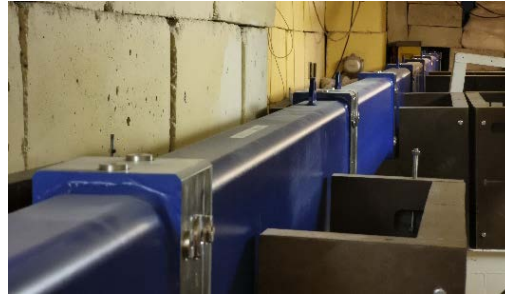
Curved part of neutron guide
